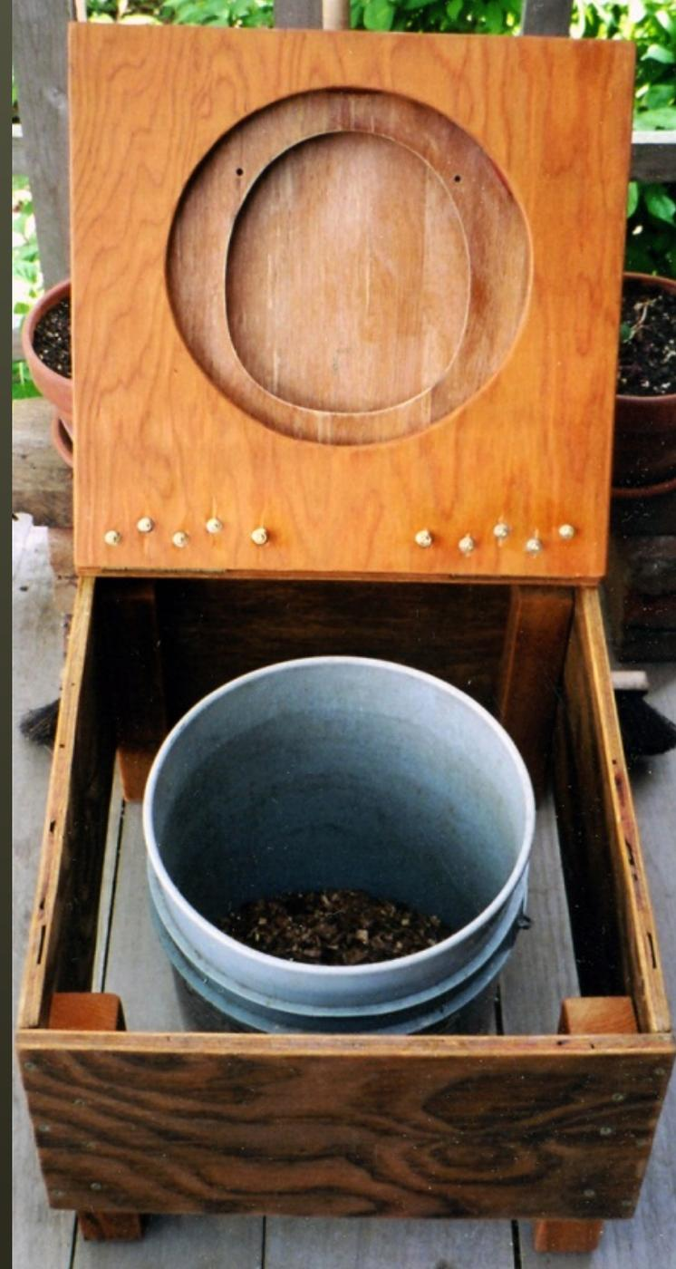
A 60 liter receptacle is about the maximum size that can be easily handled without machinery.
